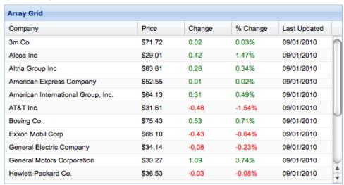
A Grid Panel displays tabular data in rows and columns. The data displayed by a Grid Panel is read from a Store. A Grid Panel's child Column components encapsulate the configuration information needed to render data into the individual columns.
