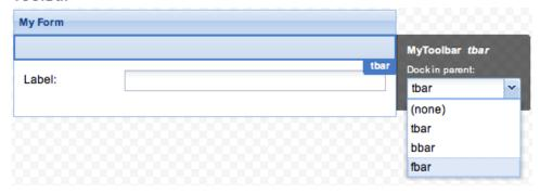
Toolbar is a container for control components such as buttons and menus.
